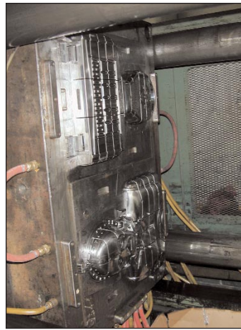
These two pictures show each side of a tool while it is attached to the press. The press pushes these two pieces together. You can see the hoses on the sides where the plastic is forced into the tool.
